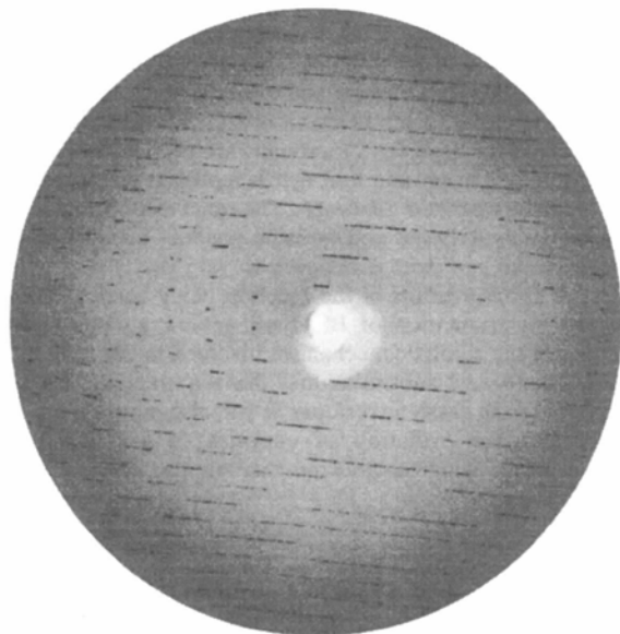
Fig. 1. An X-ray diffraction image taken at CCLRC Daresbury Laboratory on station 9.5 recorded on a large MAR image plate. The diffraction limit to the edge of the image is 3.5 Å and a rotation angle of 3^\circ was used.
